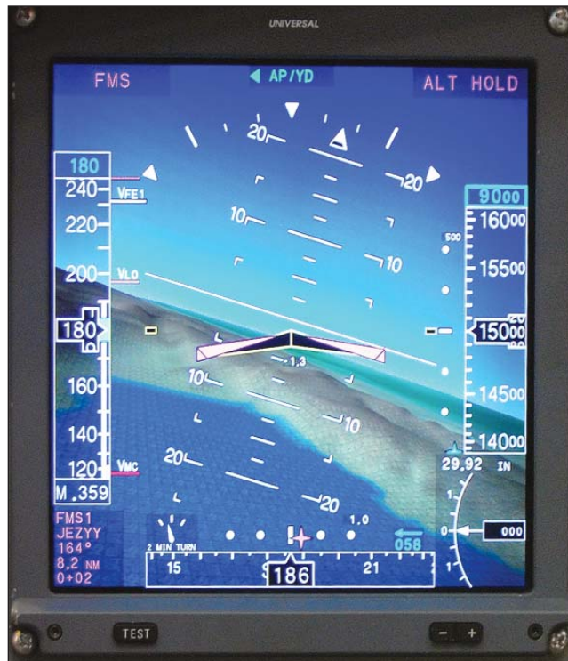
Universal Avionics Vision 1 SVS Egocentric 3D was approved by FAA in Nov 2005. Imagery depicts terrain in real time for direction of flight, including pitch and roll, while the system retains standard foreground symbology and traditional flight director cues.
