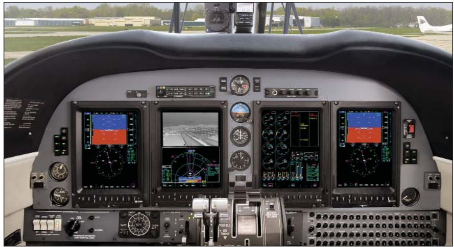
Sagem Avionics integrated cockpit display system (ICDS) upgrade in a Turbo Commander 690 with 10-in color AMLCD panels. Sagem ICDS provides primary flight instruments, engine instruments, moving maps, CAS advisories, terrain obstacle proximity system and warning/caution system. ICDS also integrates with radars and a traffic advisory system.
