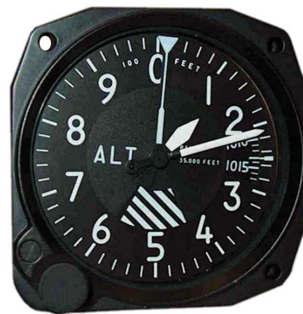
In 1928, Paul Kollsman changed aviation by inventing the world's first accurate barometric altimeter with its “Kollsman window.”
