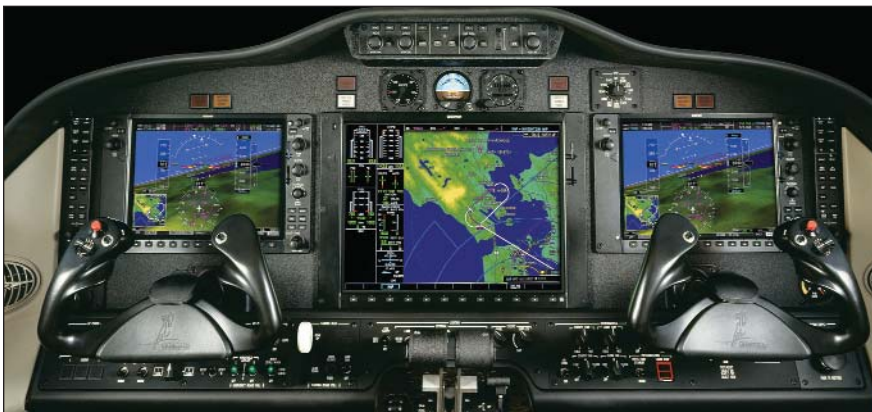
Garmin's SVT brings new levels of situational awareness to the Cessna Citation Mustang cockpit by displaying the aircraft's position on an enhanced topographical database, including SafeTaxi, which gives a graphical representation of the aircraft in the airport environment.
